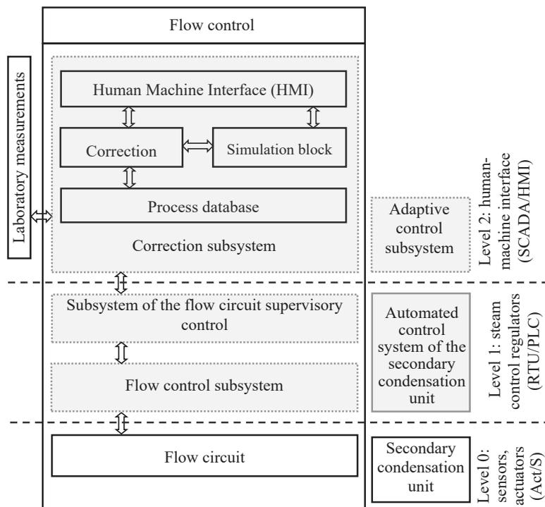
**Fig. 1.** General structure of the flow control system
