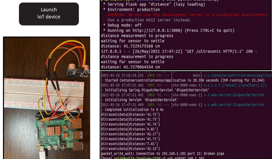
Fig. 4. Prototype of the draft IoT solution for monitoring and analysis of solid waste storage system
