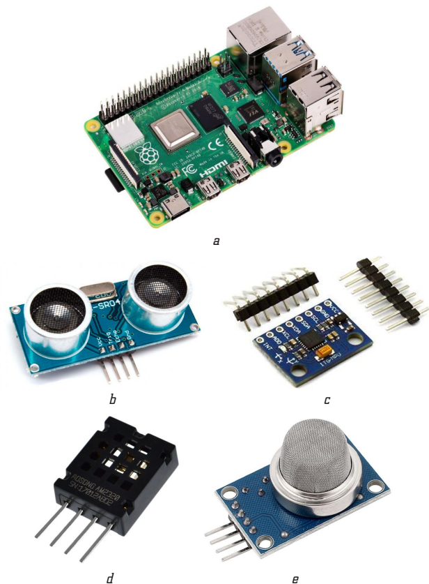
Fig. 2. Hardware support of IoT solutions for monitoring and analysis of solid waste disposal system: a – Raspberry Pi 4 Model B; b – HC-SR04; c – GY-521; d – AM2320; e – MQ-2
