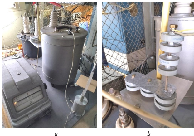
Fig. 2. General view of partial discharge: a – measuring installation; b – capacitor bank
