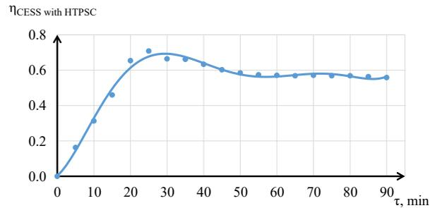
**Fig. 6.** Thermal efficiency of CESS with HTPSC  $\eta_{CESS\ with\ HTPSC}$
