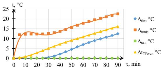
**Fig. 4.** Temperature increase of the heat carrier in the pipeline at the inlet  $\Delta t_{in}$ , °C, at the exit  $\Delta t_{out}$ , °C, from HTPSC, in TB,  $\Delta t_{TBav}$ , °C, and the ambient temperature  $\Delta t_a$ , °C
