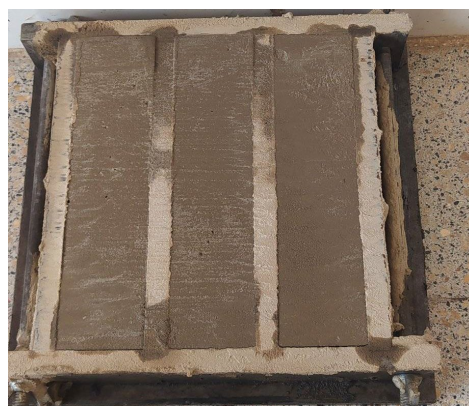
Fig. 4. Mold for making test specimens
