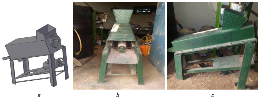
Fig. 1. The corn-cob sheller machine: a – isometric diagram; b – front view; c – side view
