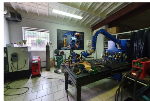
Fig. 1. Robotic WAAM system at Triada LTD Co.
