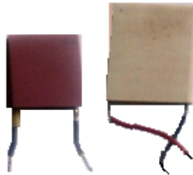
Figure 1: Single-cascade thermoelectric coolers
