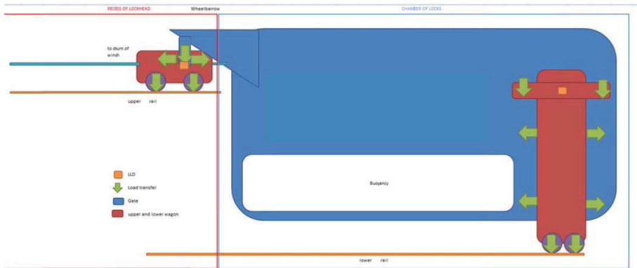
Figure 12. Conceptual diagram of the operation of the gates.
