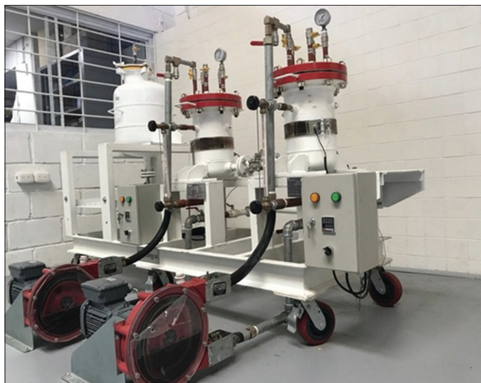
Figure 12: Reactor system implemented for the analysis of biogas production at the Universidad del Atlántico
