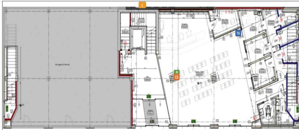
Figure 3: Virtualization of the ground floor (Legend: T=Temperature, humidity and lux measurement; C=CO 2 and temperature measurement; R=CO 2 repeater; E temperature, humidity and lux measurement outside; G=Gateway; P=Power meter)
