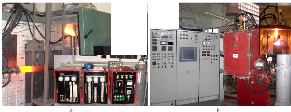
Fig. 3. General view of laboratory plasma units for the synthesis of nanosilicon for: a – 30 kW; b – 150 kW
