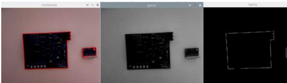
Figure 3 Object detection by contour.
