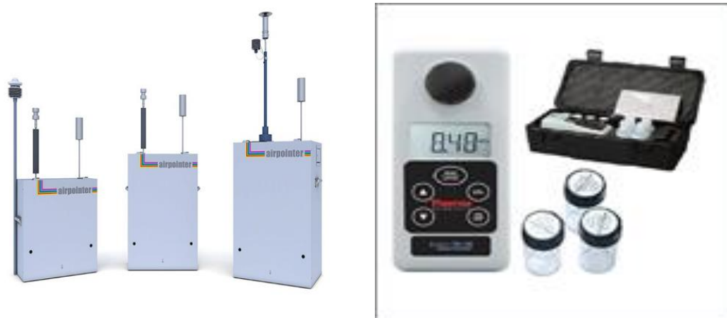
Figure 1: Air Pointer (system for air quality monitoring); Infrared Turbidimeter (designed for quick and easy turbidity measurement) (Source: https://www.znrfak.ni.ac.rs )
